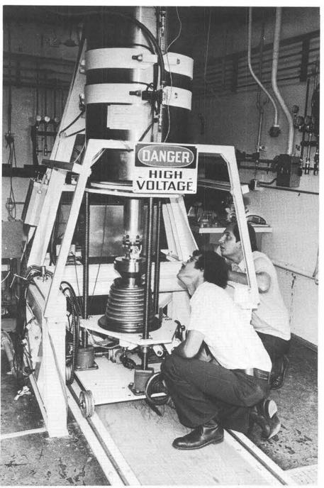
HOT STUFF - New facility in Area Y melts rock to produce magma at temperatures up to 1600°C under pressures up to 60,000 psi. Charlie Greenholt and Bob Wemple (both 5831) prepare to insert molybdenum furnace (at bottom) into the steel pressure vessel. The facility supports the Magma Energy Research Project and other materials research projects.
